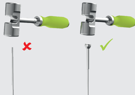
Fig. 7 Do not use a hammer with the guidewire without protection sleeve
