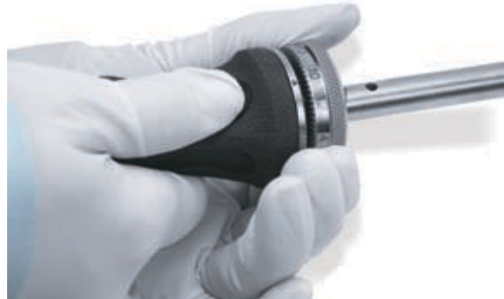
Set the appropriate torque level by turning the knurled ring
