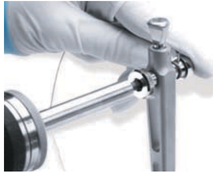
Set the appropriate torque level by turning the knurled ring
