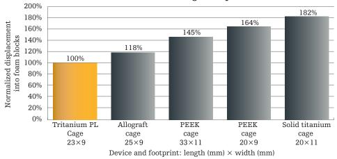
Subsidence was measured at 500 N of compressive force. Testing was performed per ASTM F2267.
