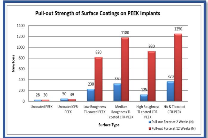
**Best in Class Pull-Out Strength (N) Properties of HA + Ti Coating** illustrated in head-to-head comparison of various coated PEEK surfaces <sup>(1)</sup>
