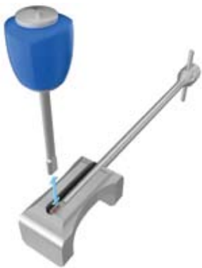
Figure 17 - Bone graft is compacted into the Cage.
