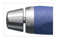
Alternatively, the **Quick Turn Screwdriver** can be used. Assemble the **Draw Rod** and Quick Turn Screwdriver. Seat the screw into the tip of the driver. The Draw Rod of the Screwdriver should protrude slightly from the handle. Thread the Draw Rod clockwise into the screw until finger tight (Fig. 11).
