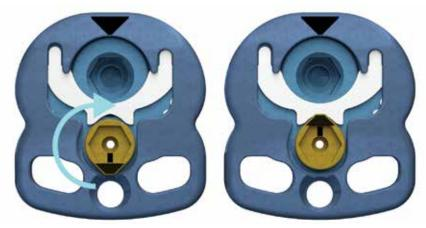
Figure 27. Locking the Plate
