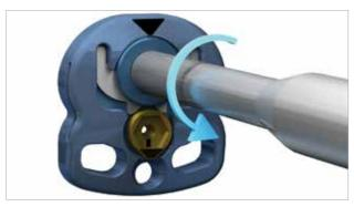
Figure 29. Removing the Screw
