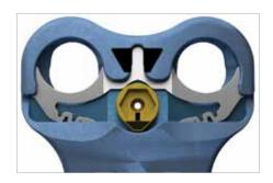
The primary screw locking mechanism is a spring-loaded bar that automatically locks over the screw heads once they are inserted into the plate. Rotation of a secondary blocker locks the bar in place for added security with visual and tactile confirmation.
