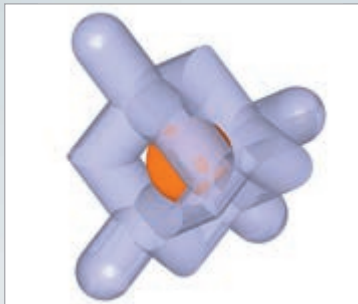
Fig. 3: Unit cell with fitted ball of 900 µm (pore size)
