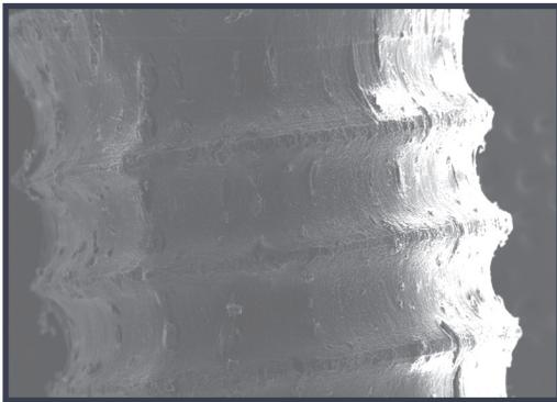
BacFast HD surface via a Scanning Electron Microscope (SEM) at a magnification of 22x.
