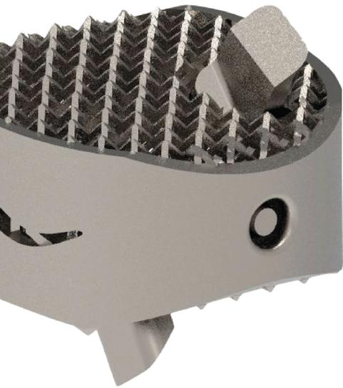
Additive manufacturing technology in combination with a unique geometrical implant design facilitates efficient and reliable primary and secondary fixation. The unique “net” structure provides strong primary fixation and eliminates the risk of implant migration. The elasticity modulus of the implant is similar to PEEK alternatives and close to natural bone characteristics, which is a key success factor of bone in-growth: secondary fixation by supporting fast and effective osteointegration.
