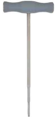
TL136106 (5.5) TL131106(6.0) Torque Limiting Final Driver (11N ± 10%)
