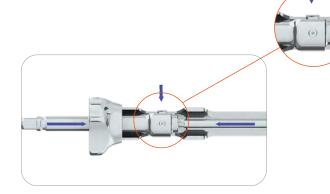
Now insert the tip of the screw driver (inner shaft) depending on the type of screw (mono/poly or reduction) into the screw head and connect the outer guide to the screw head by screwing it into the inner thread of the screw head.
