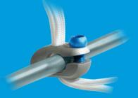
**Titanium and Stainless Steel Clamp** The clamp can be attached to a rod to reproduce native spinal curvature. Available in multiple sizes to accommodate various rod diameters: 4.5 mm (Ti); 4.75 mm (Ti); 5.5 mm (Ti & SS); 6.0 mm (Ti & SS); 6.35 mm (Ti & SS).
