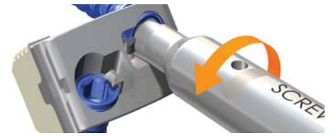
Outer sleeve rotated 180°, moving the retaining mechanism over and allowing the screw to pass
