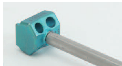
Figure 4: The Install Guide Block attaches to the end of the Inserter Tool and acts as a guide for the Awl and Bone Screws.
