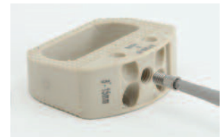
Figure 3b: The VAULT Plate is placed on the anterior face of the VAULT PEEK Cage and secured in place with the VAULT Set Screw using Torque Driver.
