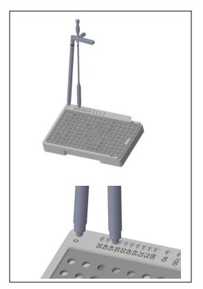
Take the locked calipers to the rod caddy of choice (either straight or curved) and place the end of one caliper arm into the dimple labeled zero. Allow the other arm to fall into whichever corresponding length dimple it aligns with.
